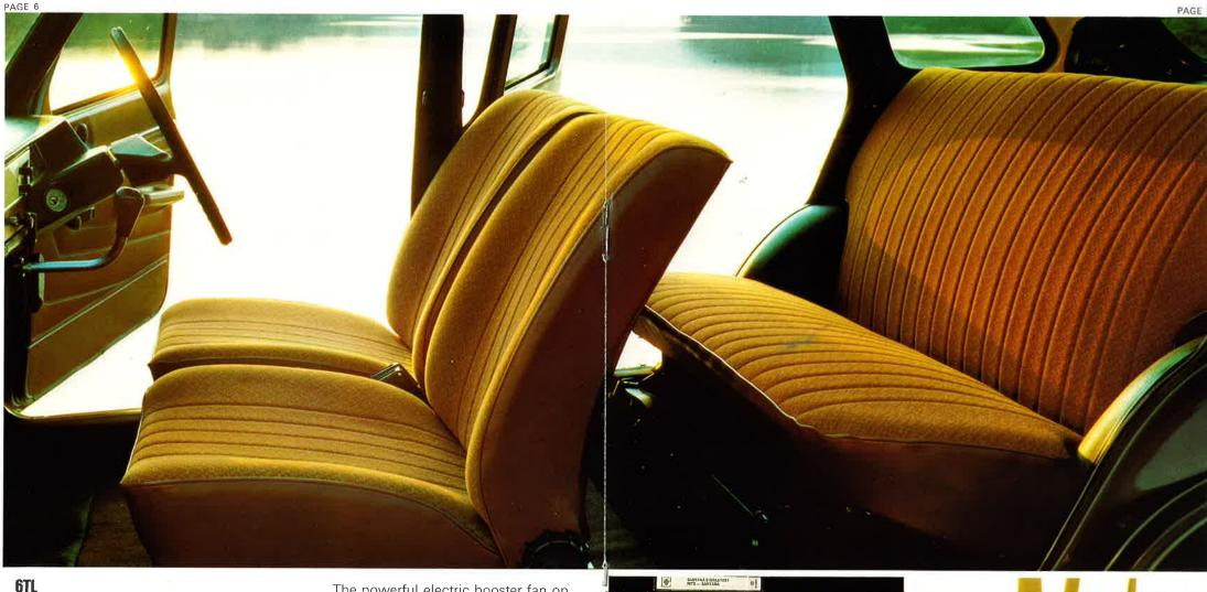
The whole family will appreciate the soft padded seats, which support each part of the body correctly according to medical experts, and harmonize with the suspension to smooth out vibrations. Covering is in soft vinyl, while cloth (as illustrated) is optional extra. The front seats are reclining and adjustable for leg room on ball-bearing runners.
